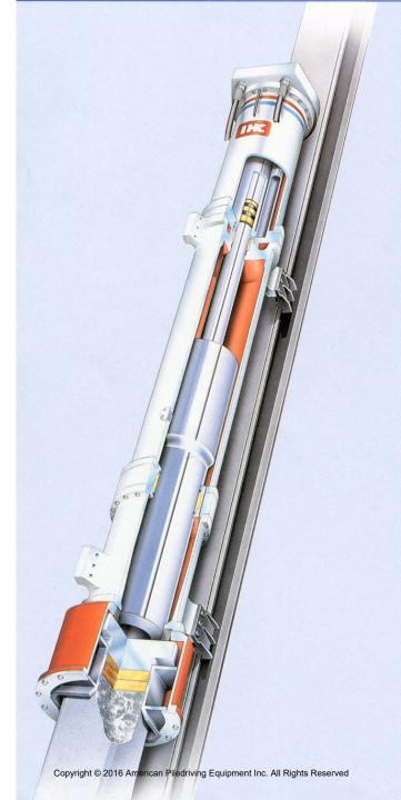
Smaller on shore hammers use hydraulic oil on down stroke
